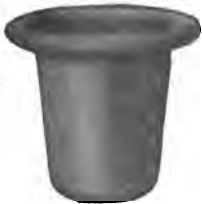
Fig. 204. Cast-Iron Pot Used for Lead Pot
